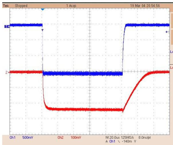
Figure 4: Pulse shape of the klystron at 350MHz
