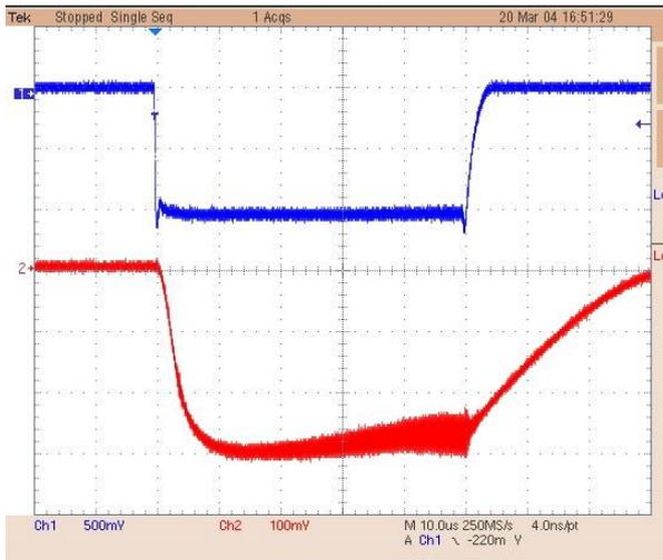
Figure 5: Pulse shape of the klystron at 352.1MHz
