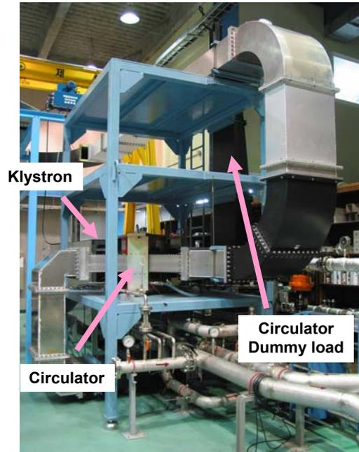
Figure 1: Klystron, circulator, dummy load
