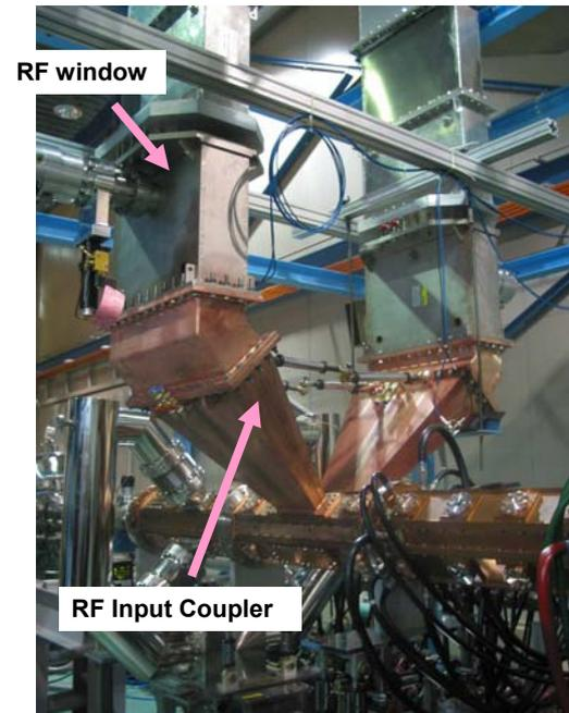
Figure 2: RF window, RF input coupler
