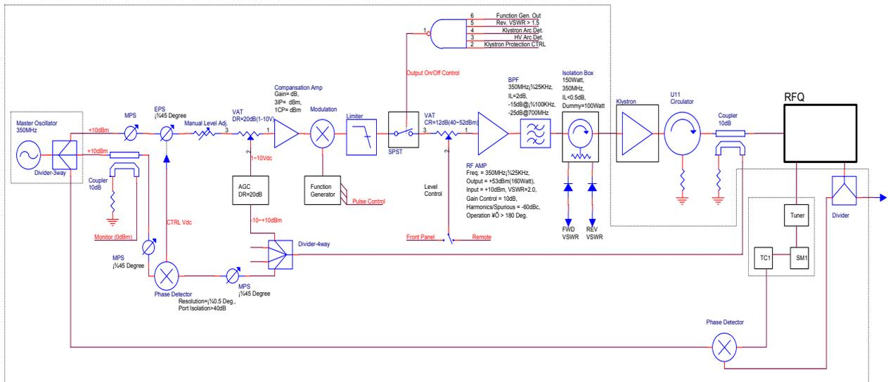
Figure 1: LLRF System Block Diagram for RFQ
