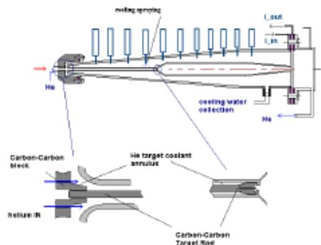
Figure 3: Proposed graphite target and horn configuration
