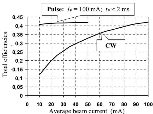
Figure 2: Dependence of complete efficiency of the linac-driver on an average beam current for continuous and pulse modes operation at RT resonators.
