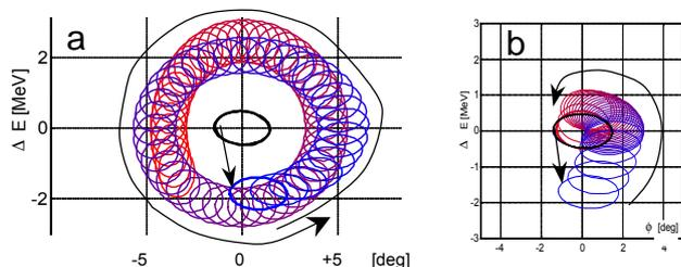
Figure 1: Evolutions of an ellipse representing a beam at switching-off of one accelerating MPA gap without indemnification (a) and with indemnification (b).
