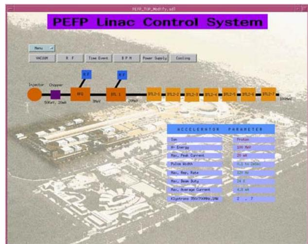
Fig. 4: Control System Architecture for the 20MeV PEFP
