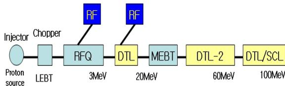
Fig. 1: PEFP Accelerator structure
