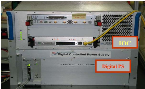
Fig. 3: MPS Control system and Digital Power Supply
