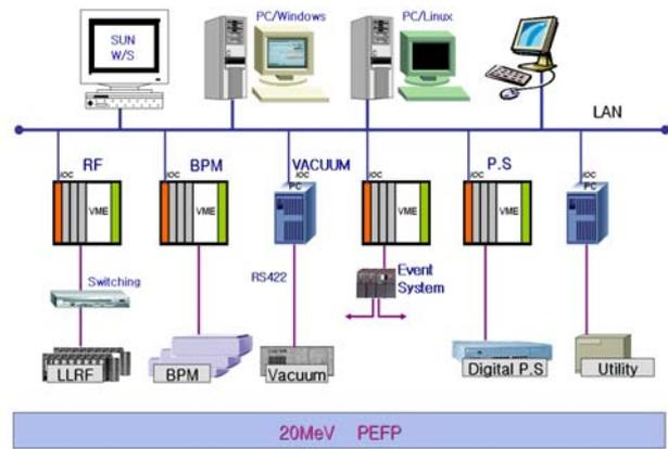
Fig. 2: Control System Architecture for the 20MeV PEFP
