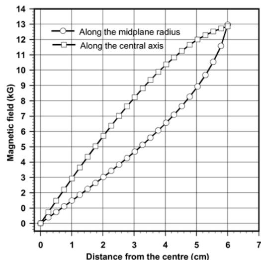
Figure 4: The computed field along the central z-axis and mid length radius i.e. the radius passing through the RCs.
