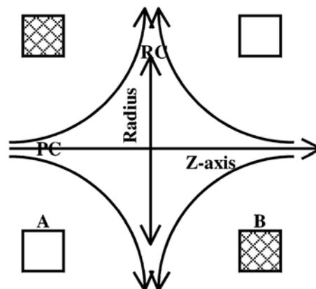
Figure 2: Scheme of simple cusp field created by oppositely energised two co-axial coils A and B.
