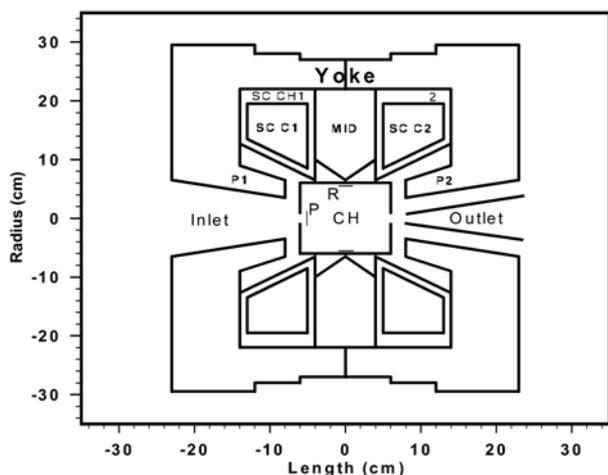
Figure 3: The geometry of the chamber CH, coils (SC C), coil chamber (SC CH), yoke, plugs (P1, P2) taken into the field calculation.
