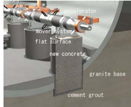
Figure 1: Layout of accelerators and stable support stands, and the cross section of stable support stand.
