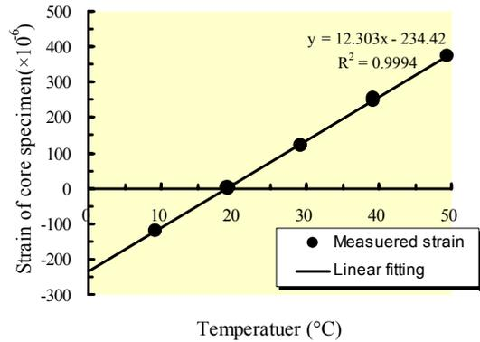
Figure 5: Relation measured core strain and temperature.
