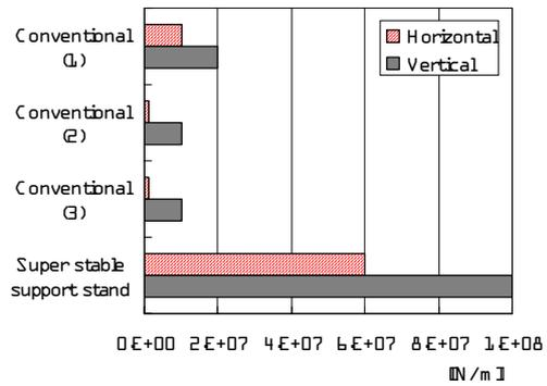
Figure 10: Measured pseudo static stiffness of the support stands.
