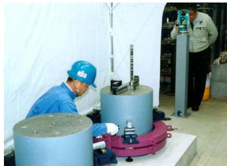
Figure 6: Adjusting alignment of support stand
