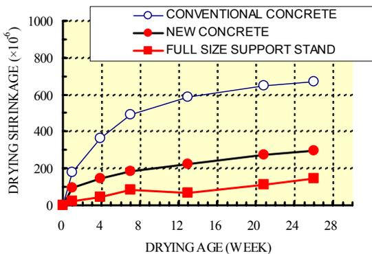
Figure 4: Test result of the relationship between drying shrinkage and drying age.
