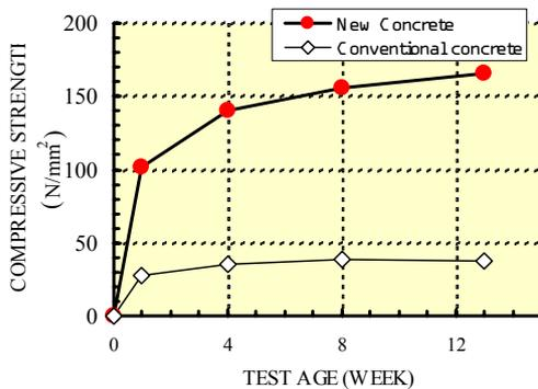
Figure 3: Test result of compressive strength.
