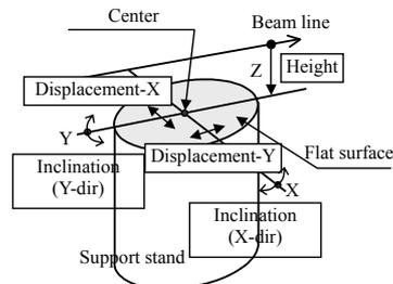
Figure 2: Alignment control direction of support stand.
