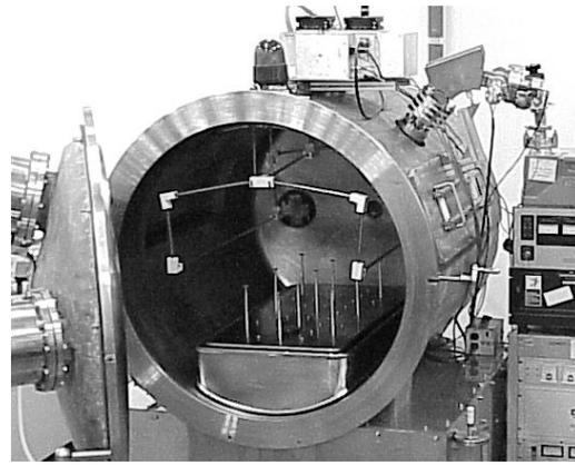
Fig. 7. Processing chamber of a 120-kV PI<sup>3</sup>D system with a 1000-liters ICP source.
