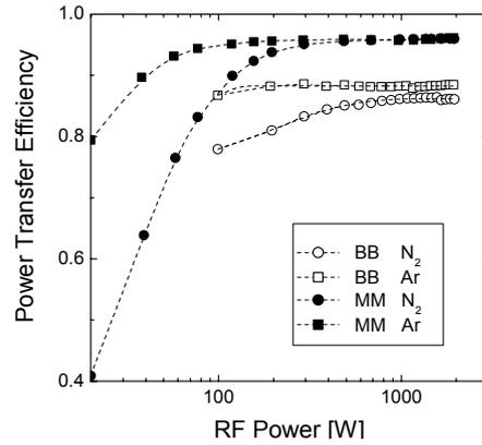
Fig. 3. Power transfer efficiency in a 100-liters and 1000-liters ICP source vs. input RF power for argon and nitrogen at pressure of 0.5 mTorr.
