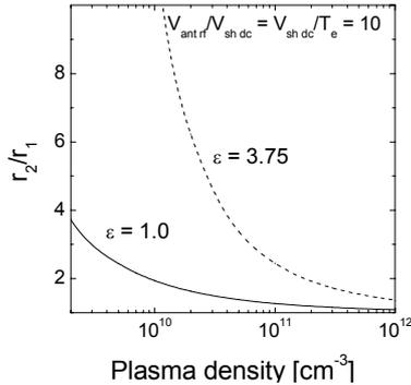
Fig. 2. Ratio of insulator – to conductor radius of the immersed RF antenna in ICP source,  $r_2/r_1$ , to obtain  $V_{=sh}/V_{rf} = 1/10$  as a function of plasma density, for air ( $\epsilon=1$ ) and quartz ( $\epsilon=3.75$ ).
