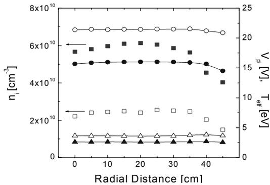
Fig. 6. Radial distribution of plasma (ion) density (squares), plasma potential  $V_{pl}$  (circles), and effective electron temperature  $T_{eff}$  (triangles) in a 1000-liters ICP source (BB) for argon at 0.2 and 1.0 mTorr (empty and filled symbols, respectively). Zero at the X-axis corresponds to the axis of a 1-m diameter cylindrical chamber.
