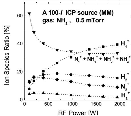
Fig. 4. Ion mass composition as a function of RF power in ammonia plasma of a 100-liters ICP source at pressure of 0.5 mTorr.
