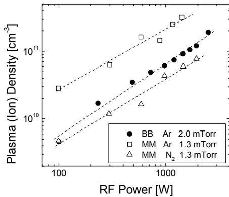
Fig. 5. Plasma (ion) density vs. input RF power in a 100-liters (MM) and 1000-liters (BB) ICP source.
