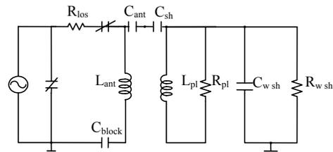
Fig. 1. Equivalent circuit of RF matching and antenna – plasma coupling in ICP source.
