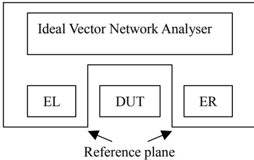
Figure 3: Error model of TRL calibration
