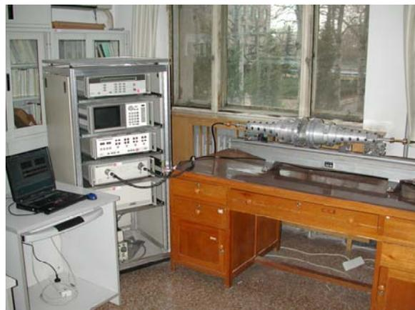
Figure 1: Layout of the longitudinal coupling impedance measurement platform
