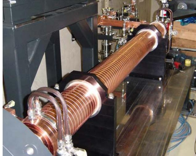
Figure 1: Photograph of the C-band accelerating structure. (1.8 m long)
