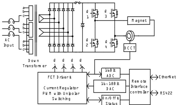
Figure 8: Structure of developed corrector MPS
