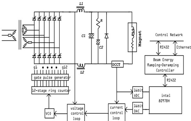
Figure 1: PLS Bending MPS structure
