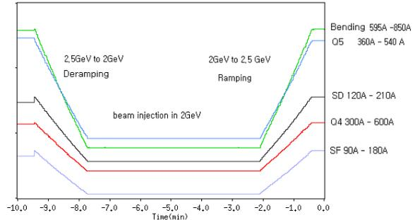
Figure 5: Uni-polar MPS Ramping, De-Ramping Current curve.
