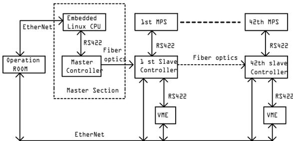
Figure 4: Digital interface controller (Uni-polar)
