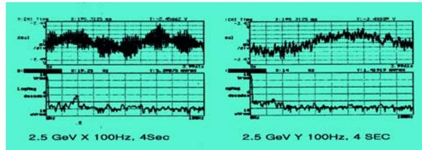
Figure 6: BPM signal before Bending MPS LC Filter change
