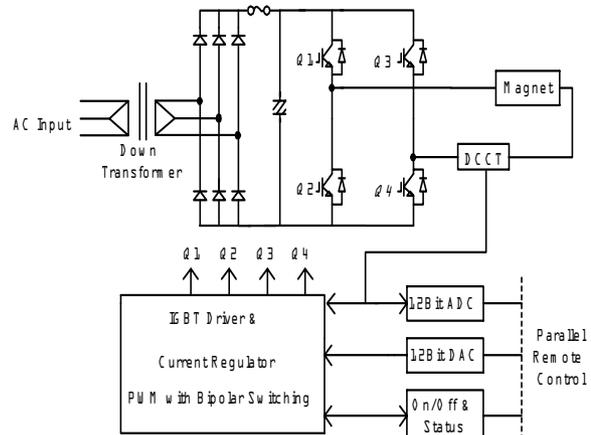
Figure 2: PLS Bipolar MPS structure
