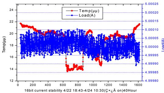
Figure 9: New corrector MPS output current stability (+6.5A: max-15A)
