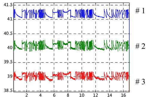
Figure 2: Temperature variations of accelerator tube at three locations, entrance, center and exit. Temperature readings at #2 and #3 are offset by -1°C and -2°C respectively for clarifying purpose.
