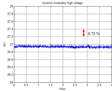
Figure 5: Long-term test of the klystron modulator high voltage after installing EMI-303L.
