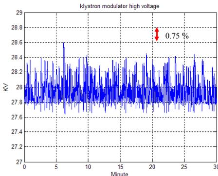
Figure 4: The variations of klystron HV modulator using resonance charging scheme.
