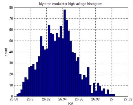
Figure 6: Long-term test of the klystron modulator high voltage histogram by EMI-303L.
