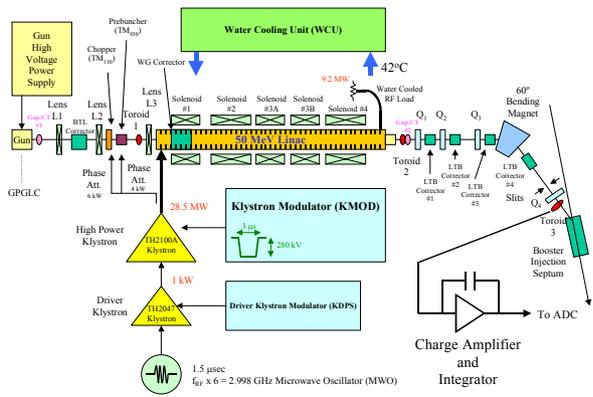
Figure 1: Synopsis of the preinjector, plus its diagnostics.
