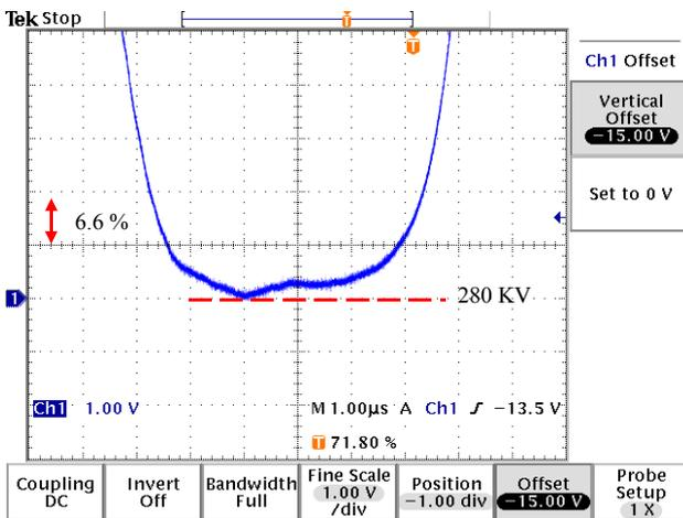
Figure 3: Typical HV pulse shape at the klystron output (offset -15V).
