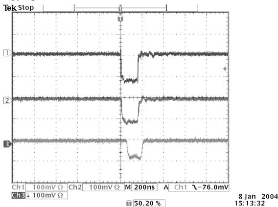
Figure 8: The signals of beam intensity monitor at linac entrance (Ch1), linac exit (Ch2), and energy slit exit (Ch3).
