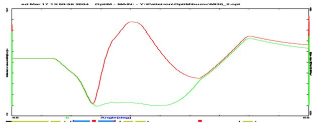
Figure 3: Beam rounding at U-bend by means of a solenoidal doublet and a single quad. The vertical scale is 1.2 cm, horizontal – 10 m.
