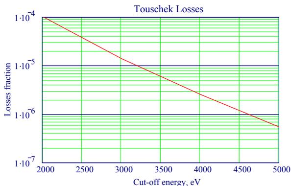
Figure 6: Touschek losses as function of the cut-off gun-collector energy, eV.
