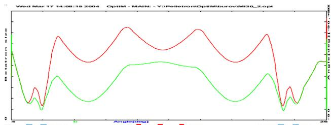
Figure 4: Invariant optics of the supply line is provided by the lattice symmetry; all the depicted quads are zeroed. The vertical scale is 1.2 cm, horizontal – 22 m.
