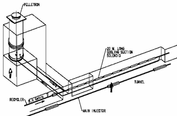
Figure 1: Schematic layout of the Fermilab electron cooler.
