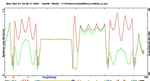
Figure 5: The beam half-axes for the whole line. The scale is 1.2 cm and 100 m.
