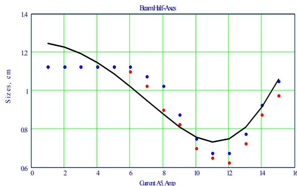
Figure 7: Beam envelope measurements (dots) and calculated best fit (line). The vertical scale is 0.6 – 1.4 cm, the horizontal – up to maximal current for the lens.
