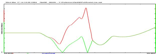
Figure 2: Beam rounding after U-bend by means of quad triplet. Green and red lines depict the 2 half-axes of the beam ellipse. The vertical scale is 1 cm, horizontal – 10 m.
