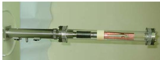
Figure 4: Photograph of a Cu photon aperture that has been melt on upper side of the aperture.
