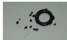
Figure 8: A damaged O-ring removed from a turbo-molecular pump located near the high radiation zone.
