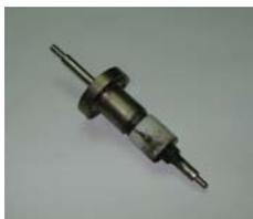
Figure 7: A feedthrough of an IP was broken by HV breakdown during the degassing of baking.
