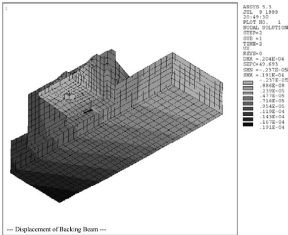
Figure 4: ANSYS result for the backing beam in the vertical (y) direction. The maximum deformation is about 20 μm if 10 metric tons of magnetic load and reaction forces from the compensation spring system are applied.
