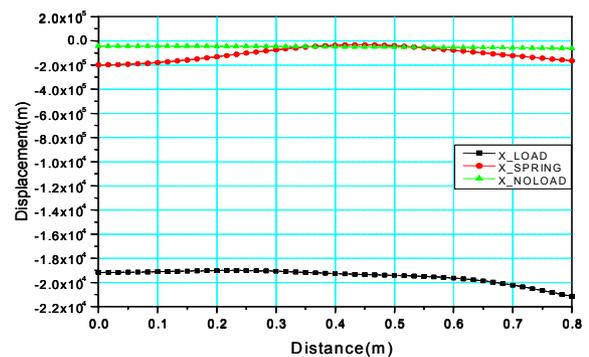
Figure 3: ANSYS result for the backing beam in the vertical (y) direction along Z-direction (beam pass) of backing beam at no load, maximum magnetic load and maximum magnetic load with reaction force.
