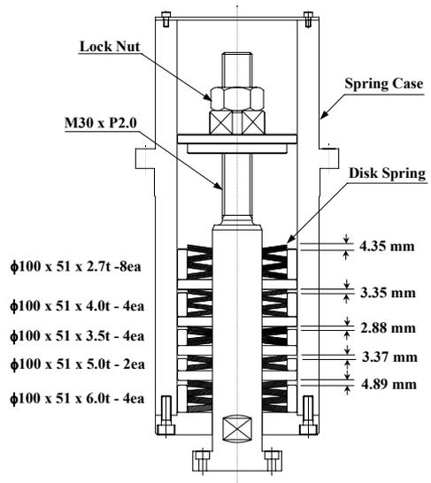
Figure 6: Design of magnetic load compensation spring system
