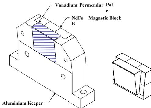
Figure 1: Geometry of the half period assembly
