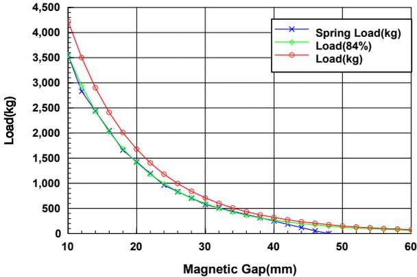
Figure 5: Magnetic load and spring load Vs magnetic gap
