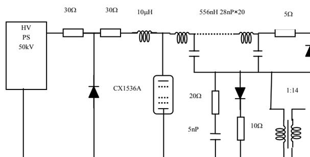
Figure 1: Diagram of The modulator
