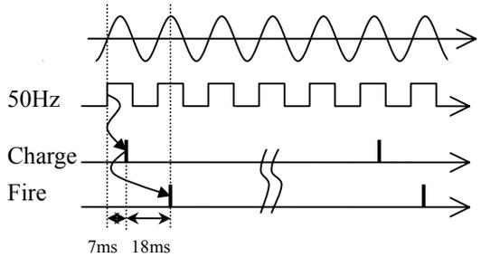
Figure 4: The time scheme for charging and firing
