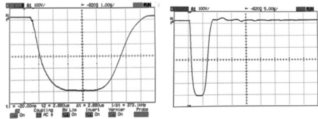
(a) Transformer output voltage waveform (309kV)
