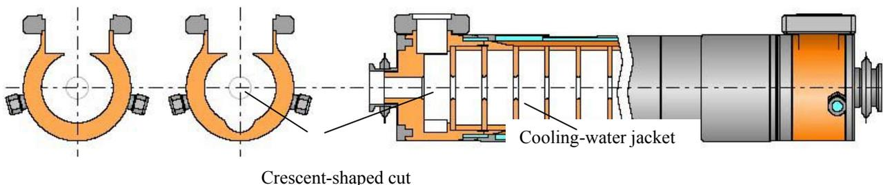
Figure 1: Cross-sectional view of the S-band 2 m-long accelerating structure.
