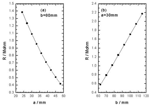
Figure 3: Shunt impedance vs cavity dimensions; (a) outer radius of the drift tube, a; (b) inner radius of the cavity, b.
