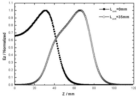
Figure 2: Distribution of the axial field with different lengths of the short drift tube.
