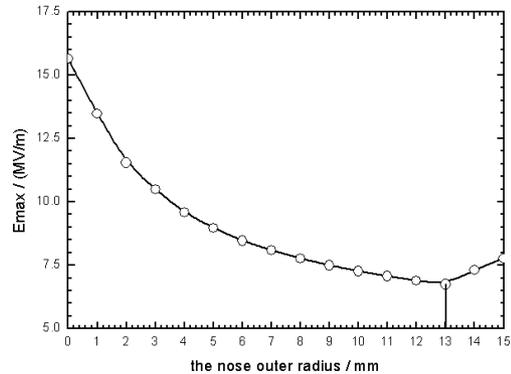
Figure 6: Maximum surface field vs the nose outer radius.
