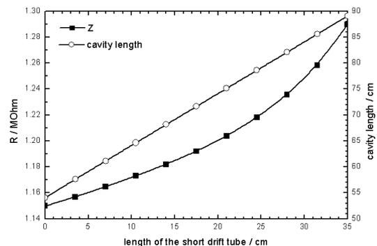
Figure 1: Shunt impedance, cavity length vs length of the short drift tube.
