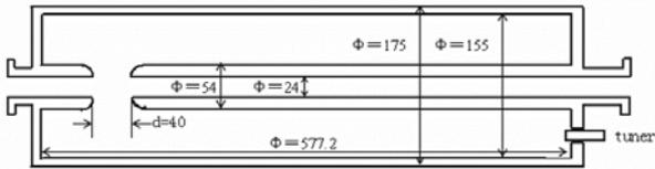
Figure 7: Structure and main dimensions of the optimized cavity (unit: mm).
