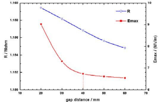
Figure 5: Shunt impedance, maximum surface field vs acceleration gap.
