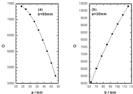
Figure 4: Q-value vs cavity dimensions; (a) outer radius of the drift tube, a; (b) inner radius of the cavity, b.
