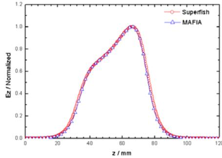
Figure 8: Comparison of the normalized axial electric field distribution.
