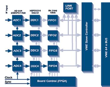
Figure 3: QDR block diagram.
