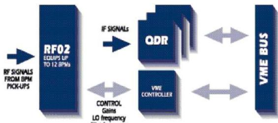
Figure 1: DBPM block diagram.
