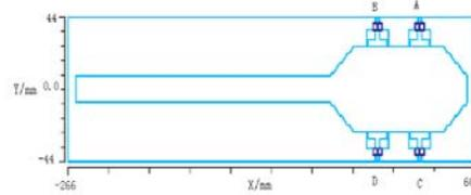
Figure 1: Transverse structure of BEPCII's BPM.
