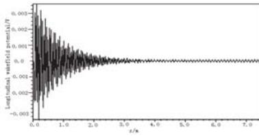
Figure 7: Longitudinal wakefield vs. particle position.
