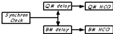
Figure 9: Phase tracking system in continuous stimulation power supply.
