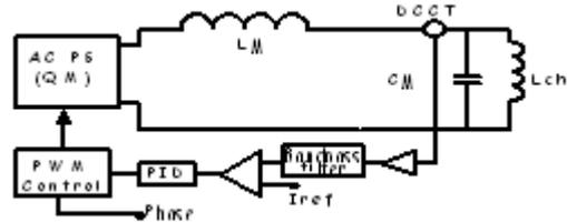
Figure 11: Continuous stimulation power supply source structure.
