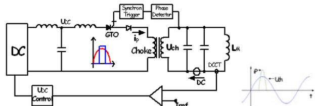
Figure 5: Single direction pulse power supply.
