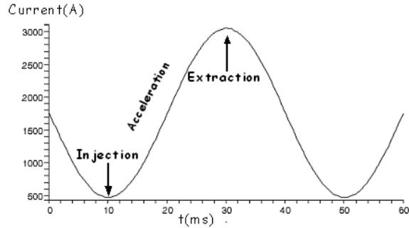
Figure 2: RCS BM current waveforms.
