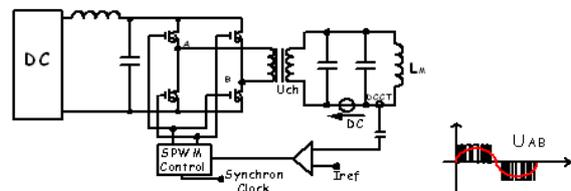
Figure 6: Continuous sinuous output power supply.
