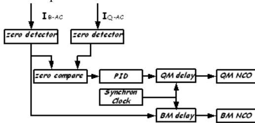
Figure 8: Phase tracking system in pulse stimulation power supply.
