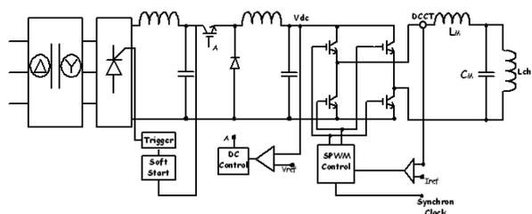
Figure 7: The scheme of ac power supply in SR network.
