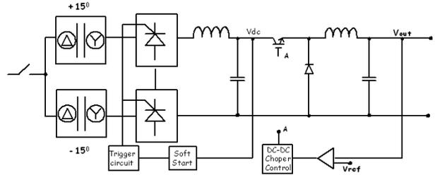
Figure 4: Simplified circuit of dc power supply.
