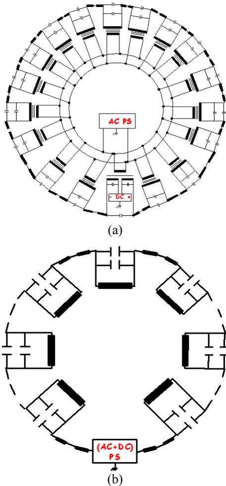
Figure 3: (a) BM Resonant Network; (b) QM Resonant Network.
