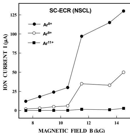
Figure 4: Variation of ion current in SC-ECR of NSCL
