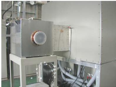
Figure 1: RF cavity and power amplifier.
