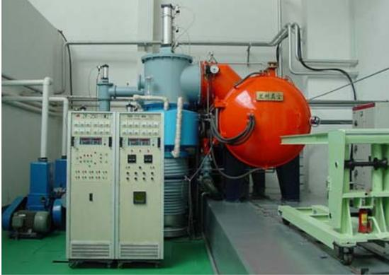
Figure 2: The large vacuum furnace
