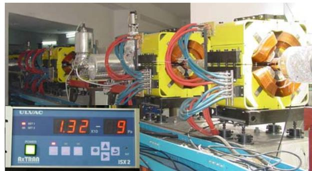
Figure 4: The vacuum system of CSR injection beam line and the pressure readings
