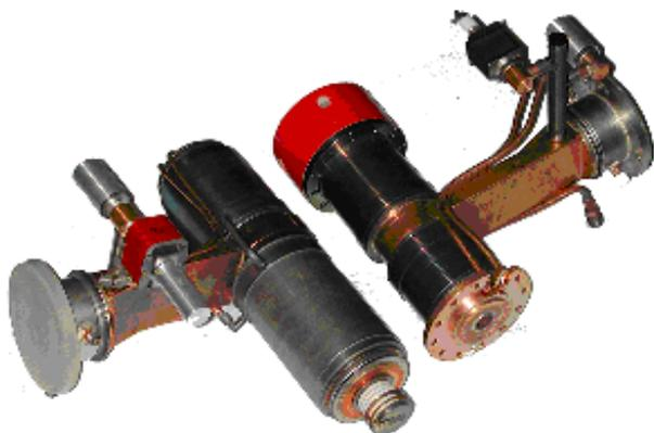
Figure 2: Photo of a 9MeV high gradient accelerating tube (down-left) compared with a 6MeV one (up-right).
