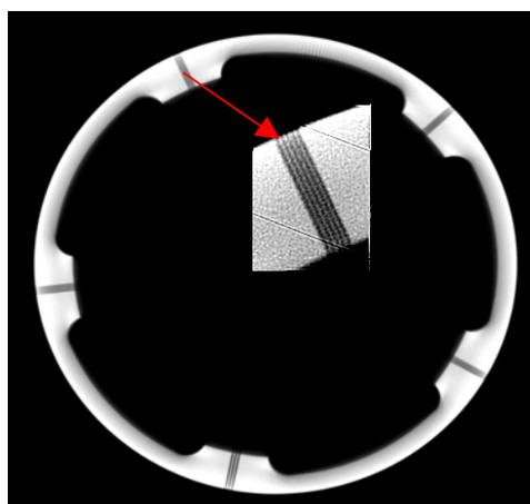
Figure 11: The CT space resolution testing picture by a ICT system with a 9MeV SW linac by CAEP.
