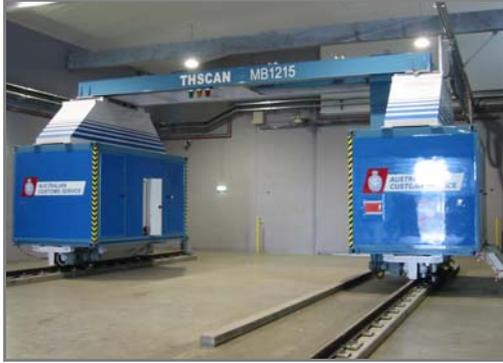
Figure 12: The 6MeV relocatable system installed in Sydney.
