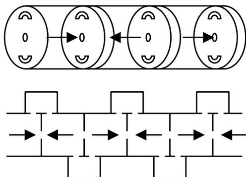
Figure 1: Accelerating structures used in medical SW linacs, magnetic on-axis coupled (up) and side-coupled (down).
