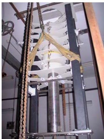
Figure 9: The 10MeV radiation processing travelling wave accelerating waveguide.
