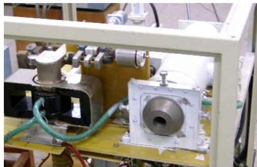
Figure 10: The X-band travelling wave mini linac by Nanjing University.
