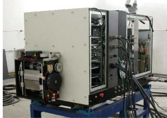
Figure 15: The 9MeV linac HEXTRON-3000 for NDT developed by Tsinghua and NUCTECH.
