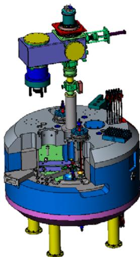
Figure 6: Main structure of CYCIAE-10.
