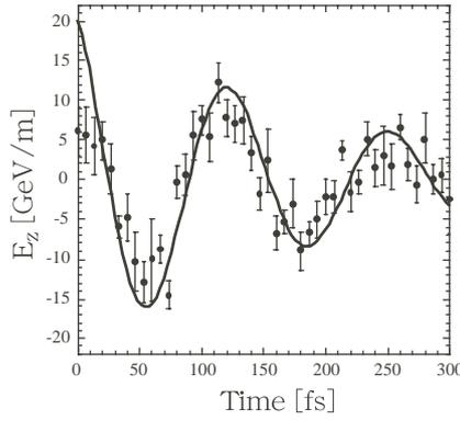
Figure 2: The longitudinal wakefield amplitude measured at the laser intensity  $I = 8.4 \times 10^{17} \text{ W/cm}^2$  ( $a_0 \approx 0.6$ ) and the electron plasma density  $7 \times 10^{17} \text{ cm}^{-3}$  with the frequency domain interferometer in a gas jet plasma. The solid curve shows a fit of the wakefield with oscillation period of 130 fs.
