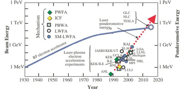
Figure 3: Evolution of the electron beam energy frontier of the RF electron accelerators (solid line) and the maximum electron energy plots achieved by the worldwide laser and plasma accelerator experiments. The dotted line shows evolution of the focused laser intensities represented by the ponderomotive energy.
