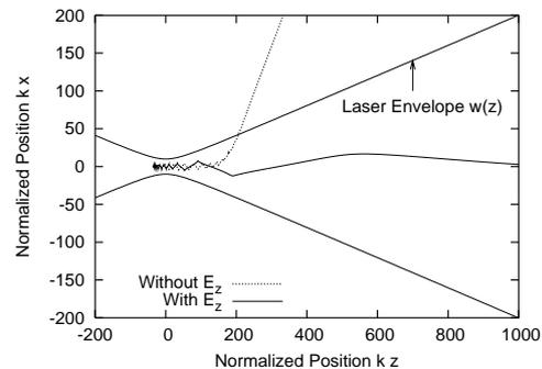
Figure 1: Typical trajectories of an electron accelerated by the fundamental Hermite-Gaussian mode, TEM<sub>00</sub>, with the peak laser field  $a_0 = 10$  for the cases with and without the longitudinal electromagnetic fields.
