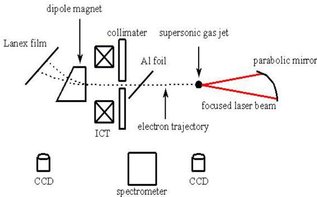
Figure 2: Schematic of the experimental setup for the self-modulated laser wakefield acceleration.
