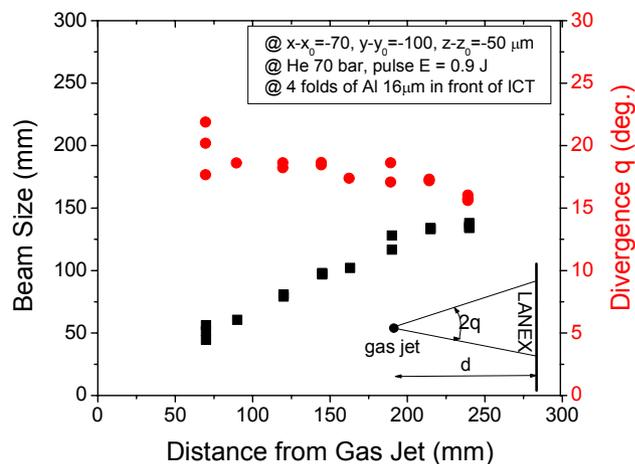
Figure 5: Measurement of a beam size as a function of the distance from the gas jet.
