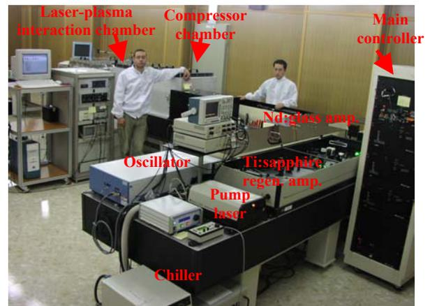
Figure 1: Overall picture of the laser system.
