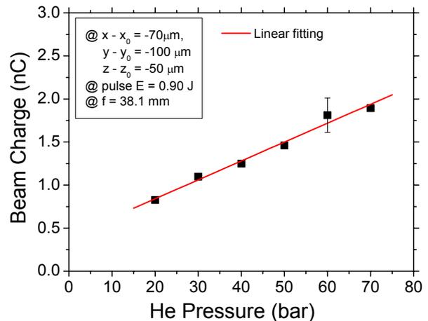
Figure 4: Electron beam charge as a function of the He backing pressure. This result implies that the beam charge is linearly proportional to the plasma density.
