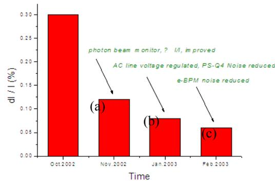
Figure 3: The reductions in photon beam fluctuations. Improvements of I<sub>0</sub> monitor (a), ripples reduction in Q4 power supply (b), and in electron BPMs (c).
