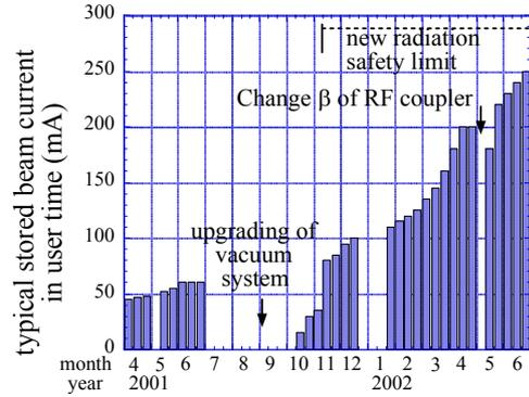
Figure 3: Increase of the typical stored beam current during the user time.
