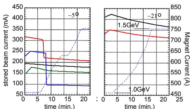
Figure 5: The stored beam current with the tuning angle of  $-5^\circ$  (left plot) and  $-21^\circ$  (right plot). The broken lines are current of bending magnet (right axis). The solid lines are examples of stored beam current (left axis) during the acceleration. The beam had been lost by the horizontal TM110 HOM.
