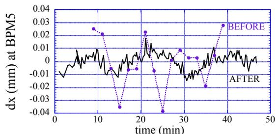
Figure 6: Improvement of the drift of the horizontal beam position by the stabilization of the cooling water temperature from  $\pm 1.5$  degrees to  $\pm 0.5$  degrees. The BPM15 is one of beam position monitors set at the dispersive sections.
