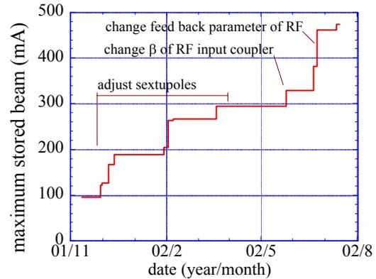
Figure 4: Improvement of the maximum stored beam current. The maximum current was limited to 500mA by the radiation safety condition at the present.
