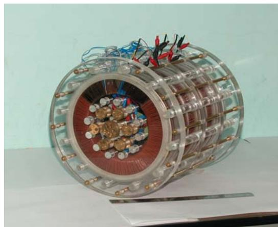
Figure 2: Amorphous core based Pulse Transformer
