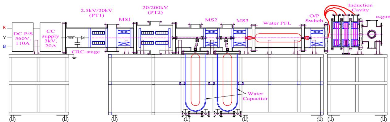
Figure 1: Schematic of Linear Induction Accelerator (200keV, 5kA, 100ns, 10-100Hz)
