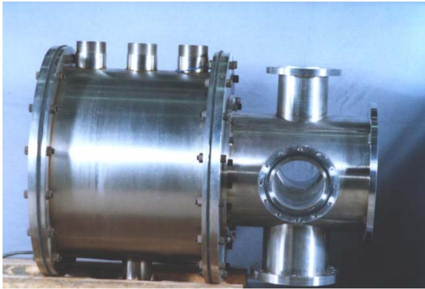
Figure 3: Three-stage Induction ADDER with gun chamber
