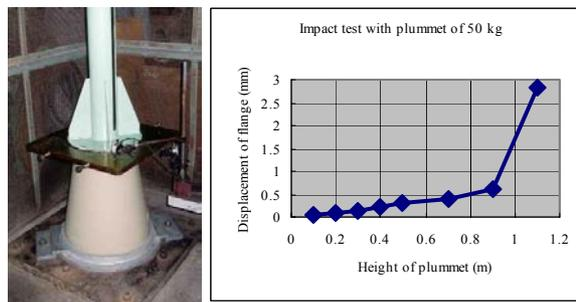
Figure 6: Setup and results of the impact test.
