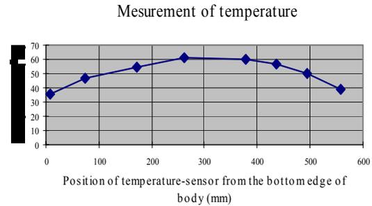
Figure 3: Temperature versus position of temperature-sensor from the bottom edge of the heated body.
