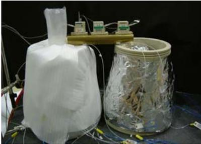
Figure 2: Setup of expansion rate measurement.
