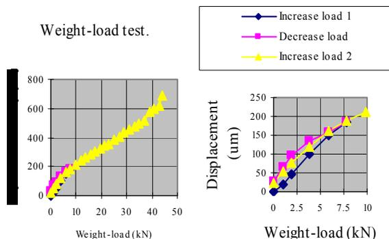
Figure 5: Results of the weight-load test. Left-hand-side: Displacement of the flange versus weight-load. Right-hand side: A zoom of the left-hand side plot.
