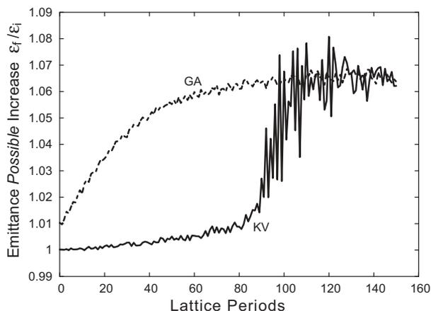
Figure 3: Possible emittance increase during the final beam bunching at initial KV and GA distributions.
