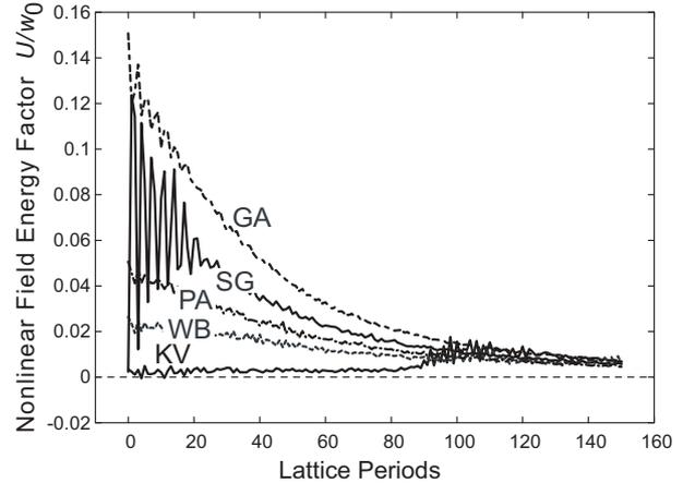
Figure 2: Nonlinear field energy factor during the final beam bunching at various initial distributions.
