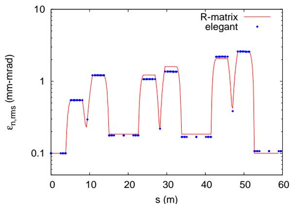
Figure 5: Beam emittance calculated by R-matrix and elegant.
