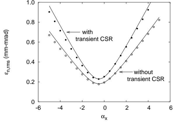
Figure 3: CSR-induced projection emittance growth with scanning the beam envelope calculated by R-matrix (solid lines) and particle tracking (dots).
