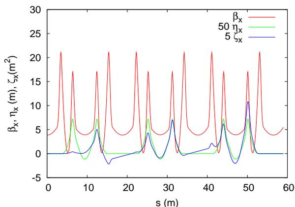
Figure 4: Beam envelopes for a series of TBA cells, where the betatron phase advance for a single cell is  $\Delta\psi_x = (8/3)\pi$ .
