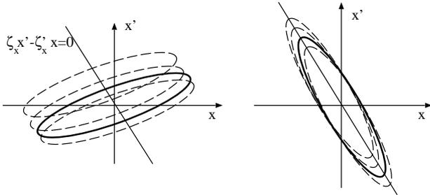
Figure 2: Two-dimensional phase ellipse in the  $(x, x')$  plane, and displacement of bunch slices due to the CSR kick. Two cases for large emittance growth (left) and small emittance growth (right).
