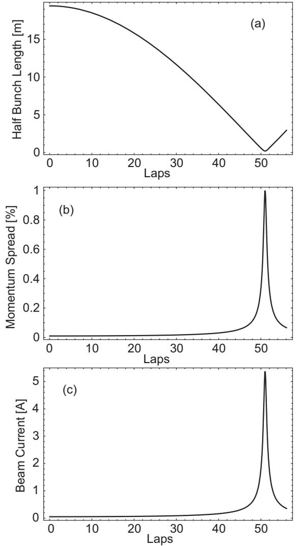
Figure 2: Longitudinal beam behavior as a function of revolution laps during bunch compression in ring, (a) half bunch length, (b) (incoherent) momentum spread, and (c) beam current, respectively.
