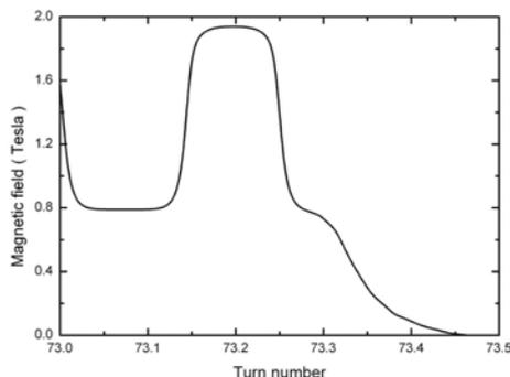
Figure 3: The magnetic field around the carbon foil and after stripping
