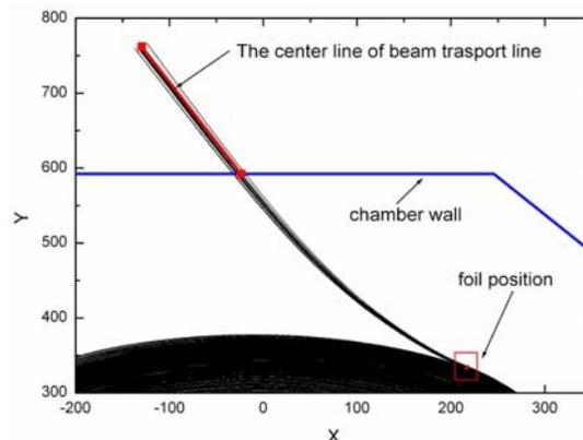
Figure 4: Beam trajectories in horizontal motion
