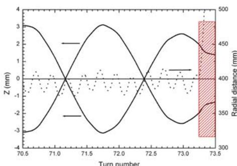
Figure 2: Vertical motion and radial distance from the cyclotron center. The inner rectangular box represents the region after stripping.
