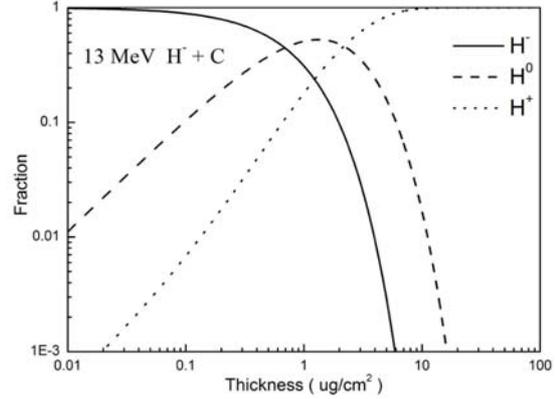
Figure 1: The calculated charge fractions of H
