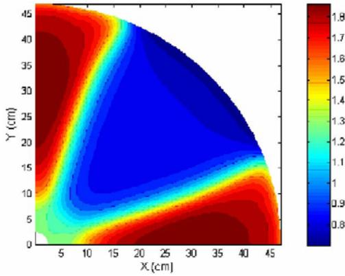
Figure 4: Measured magnetic field map.
