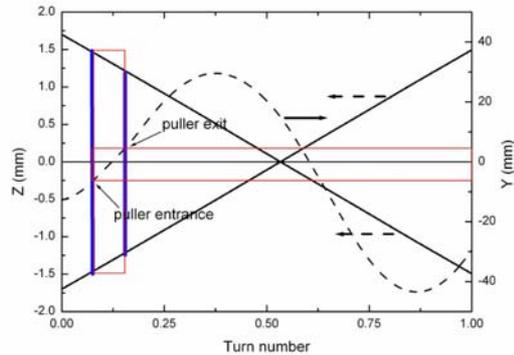
Figure 7: The vertical motion during one turn. The left axis means the vertical displacement, and the right axis the y-coordinates of the beam position.
