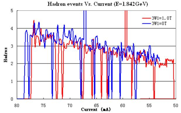
Figure 5: The hadron events rate vs. beam current in the parasitic mode and normal colliding mode.
