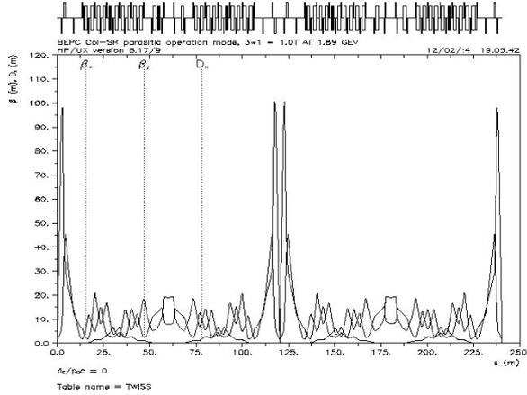
Figure 1: The lattice of the parasitic mode.
