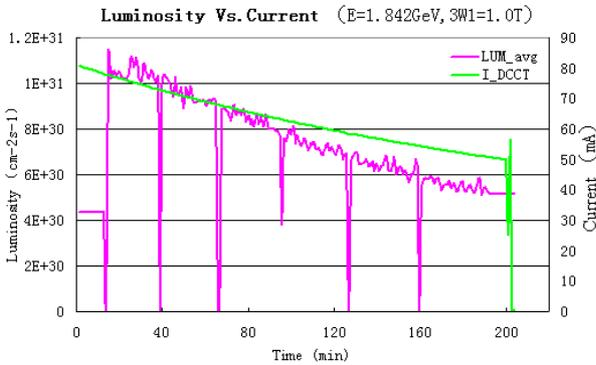
Figure 3: The luminosity vs. beam current for the parasitic mode (E=1.842GeV).
