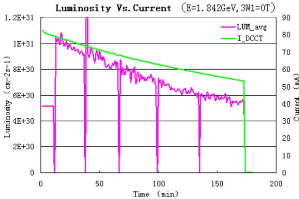
Figure 4: The luminosity vs. beam current for the colliding mode (E=1.842GeV).
