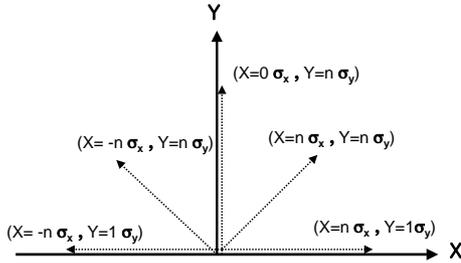
Figure 1: Survey of the dynamic aperture in the  $X - Y$  plane. The dynamic aperture is obtained by averaging these five points.
