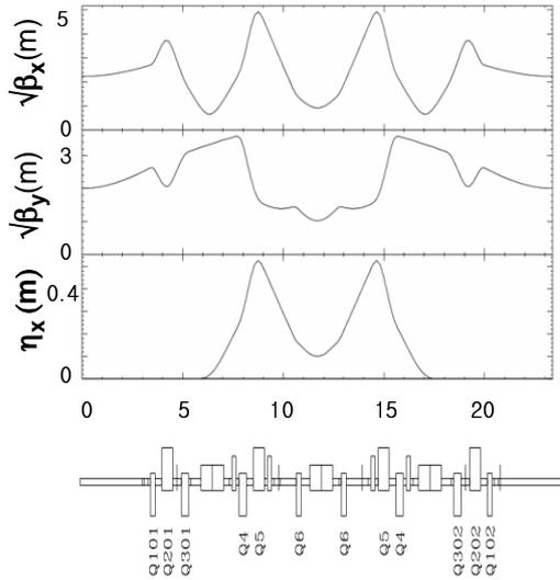
Figure 2: A low emittance lattice with emittance of 10.3 nm at 2.5 GeV.
