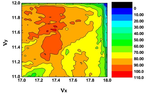
Figure 3: Dynamic apertures for tune survey in a low emittance lattice without machine errors. Most tunes show larger dynamic apertures than 70.
