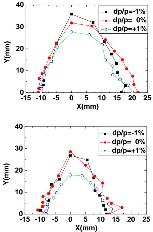
Figure 4: Dynamic apertures in the tune of  $\nu_x = 17.64$  and  $\nu_y = 11.6$  at the position of straight section. (a) without machine errors and (b) with machine errors and after corrections of the COD in (a).
