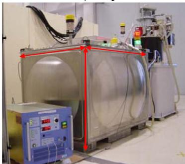
Figure 3: A new developed oil filled modulator.
