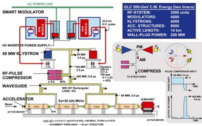
Figure 1: One unit of the C-band main linac.
