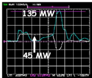
Figure 4: Typical pulse compressor cavity rf power waveforms.
