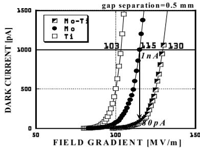
Figure 5: Dark currents for Mo-Ti, Mo-Mo, and Ti-Ti electrodes as a function of field gradient at the cathode surface with a gap separation of 0.5-mm.
