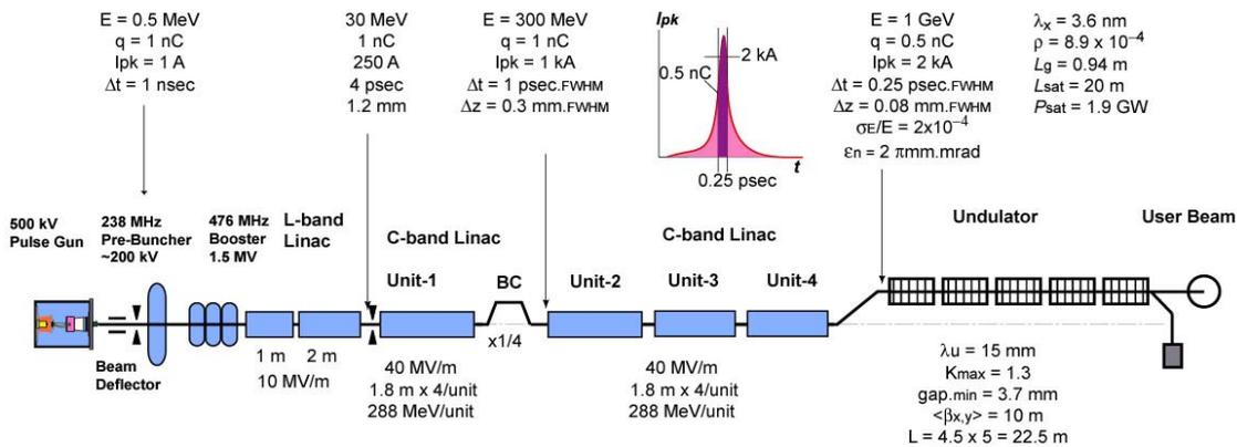
Figure 6: Beam line layout in SCSS of 1-GeV case.
