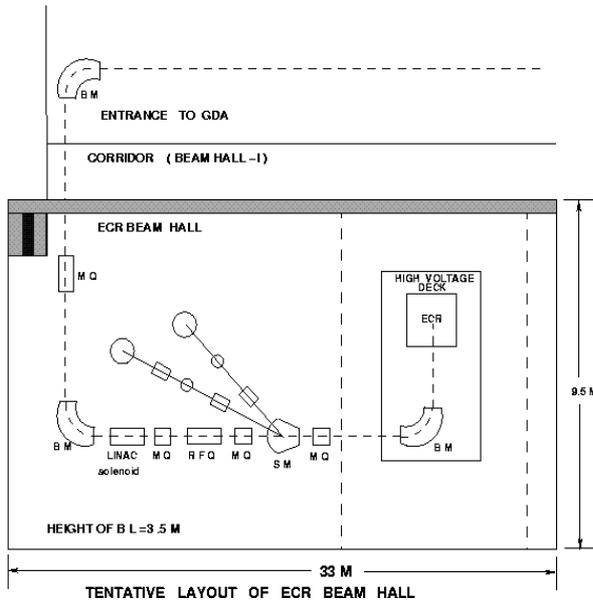
Figure 5: Layout of beam hall for the high current injection into superconducting linac
