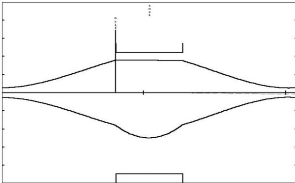
Figure 1: First order calculation (using TRANSPORT, upper: non- dispersive plane, lower: dispersive plane)
