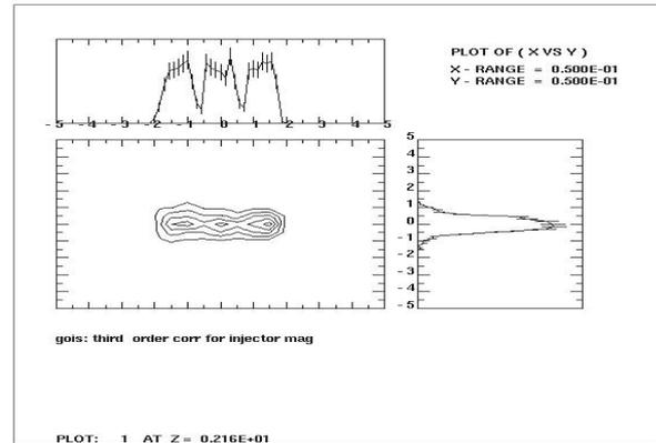
Figure 2: Third order calculation with correction, mass dispersion of 1.5 %, using GIOS [7]
