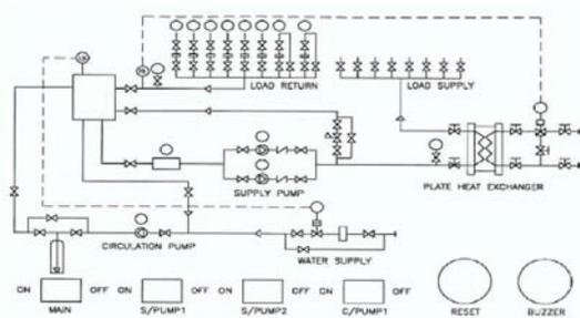
Figure 3: Diagram of Cooling System[2]
