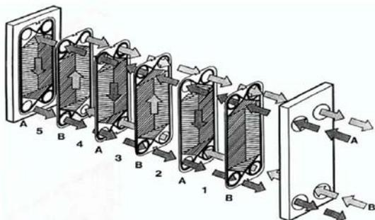
Figure 4: Schematic of Plate Heat Exchanger
