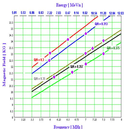
Fig. 2 Operating diagram where dots represent the beams developed
