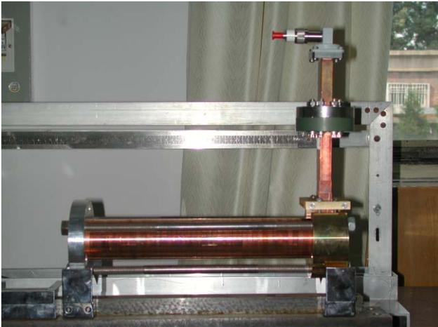
Figure 3: accelerating tube (with waveguide)
