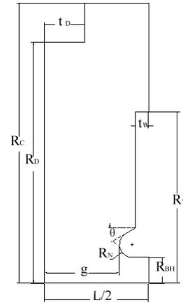
Figure 4: Geometrical parameters of a half-cell DAW cavity
