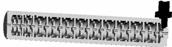
Figure 5: cutaway view of accelerating tube
