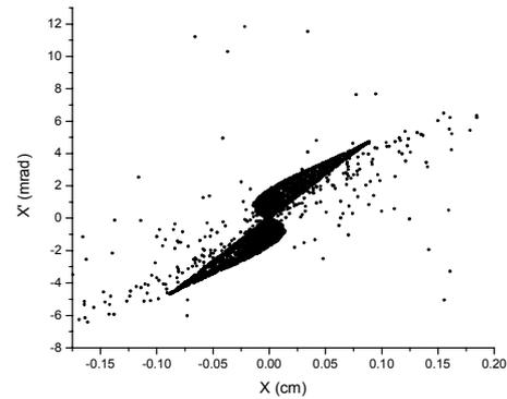
Figure 7(b): phase space distribution of emission electron
