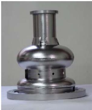
Figure 4: Image of the 1+1/2 cell niobium cavity.
