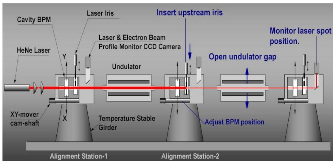
Figure 5: Laser alignment system for the undulator line.
