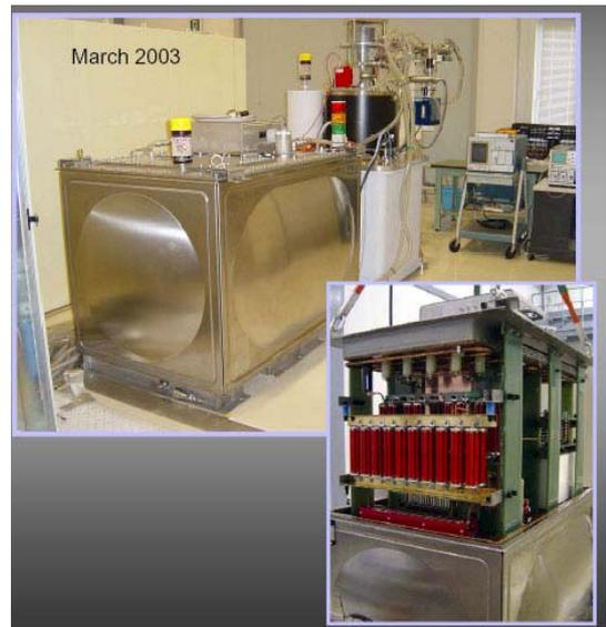
Figure 4: Pulse power modulator for the 50 MW C-band klystron, and the 500 kV electron gun.
