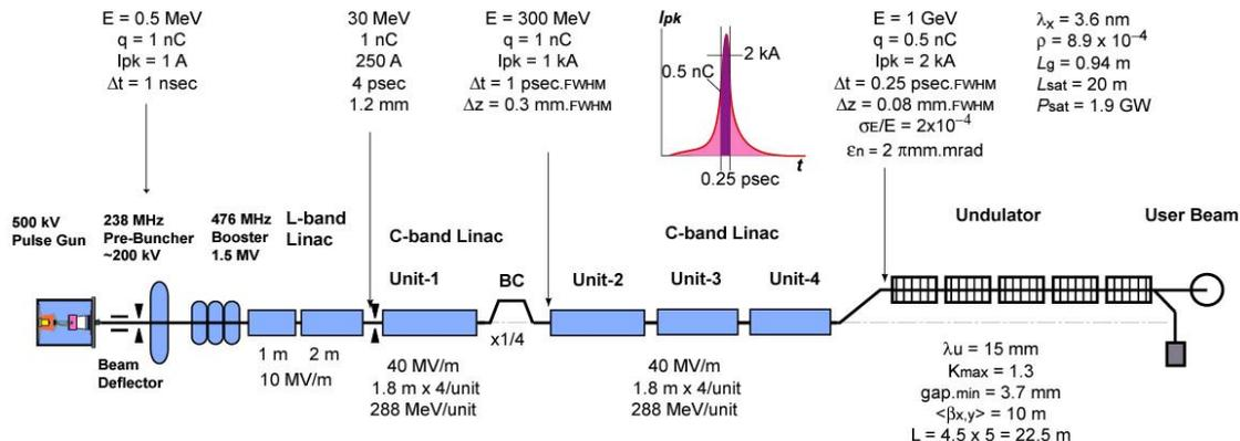
Figure 1: Beam line layout in SCSS of 1 GeV case.
