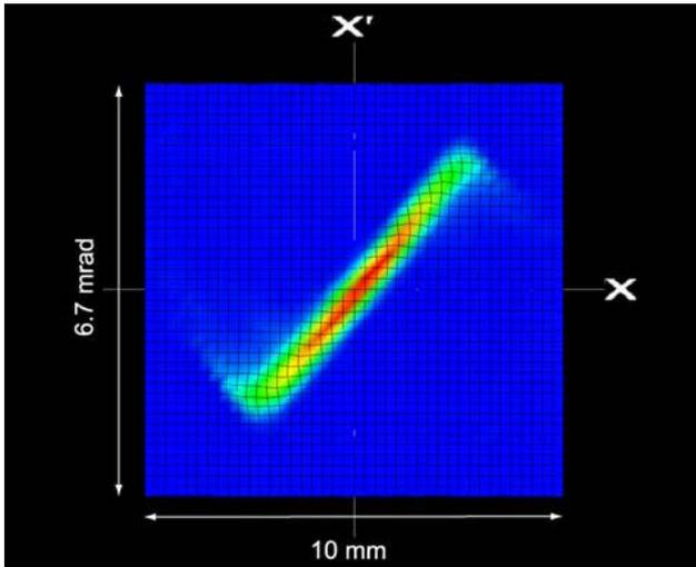
Figure 3: Phase space plot ( $x, x'$ ) of the measured electron beam at 500 kV, 1 A current. The slice time is 5 nsec, and full pulse length is 3 micro-sec.
