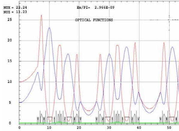
Figure 2: Lattice functions of a half SSRF super-period
