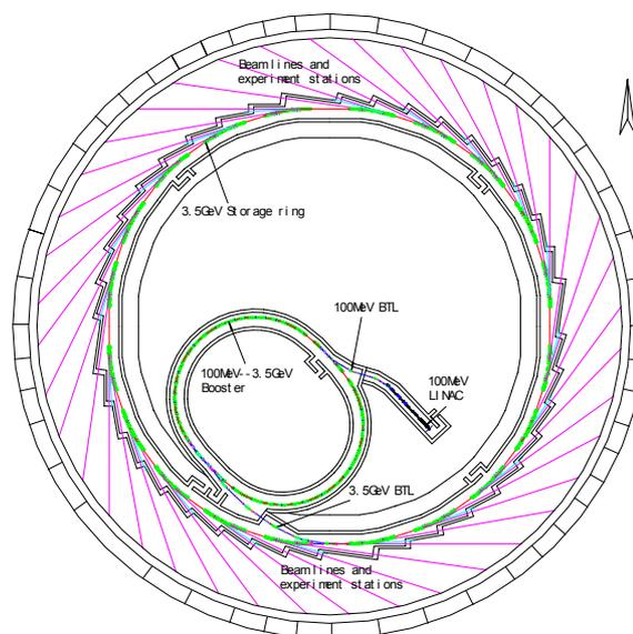
Figure 1: Layout of the SSRF
