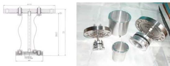
Figure 3: The detector structure for EC measurement.
