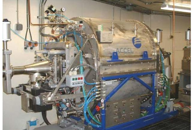
Figure 3: CLS Superconducting RF cavity.
