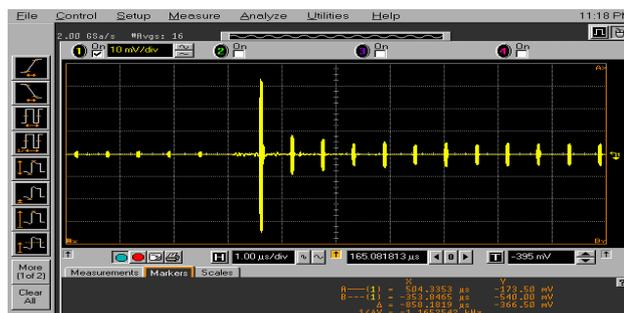
Figure 4: First stored beam at CLS.
