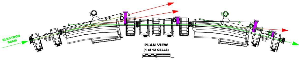
Figure 2: Layout of a single storage ring cell.
