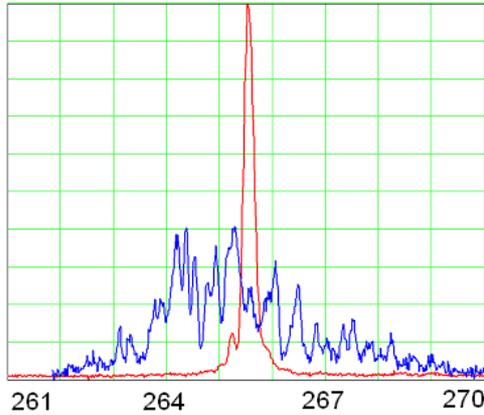
Figure 4: Single-shot HGHG spectrum exhibiting a 0.1% FWHM bandwidth (red curve). Blue curve represents SASE spectrum (magnified by the factor of  $10^5$ ). Horizontal axis is scaled in nanometers.
