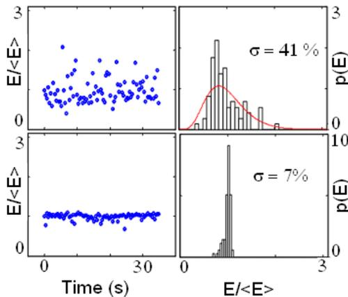
Figure 5: Time dependence and histograms of HGHG and SASE output pulse energies.
