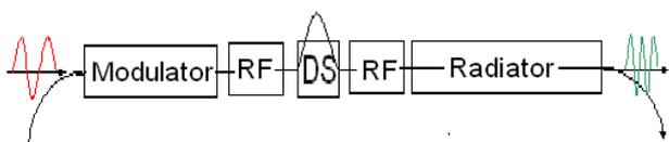
Figure 2: Dedicated scheme for the tuneable HGHG FEL. RF sections are located before and after dispersive section locally providing the energy chirp required for the wavelength compression.
