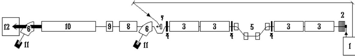
Figure 3: The DUVFEL layout. 1 – gun and seed laser system, 2 – RF gun, 3 – linac tanks, 4 – focusing triplets, 5 – magnetic chicane, 6 – spectrometers dipoles, 7 – seed laser mirror and electron beam local bump, 8 – modulator, 9 – dispersive section, 10 – NISUS wiggler (radiator), 11 – beam dumps, 12 – FEL user experimental area.
