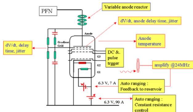
Figure 3: Experimental setup for the thyatron R&D.
