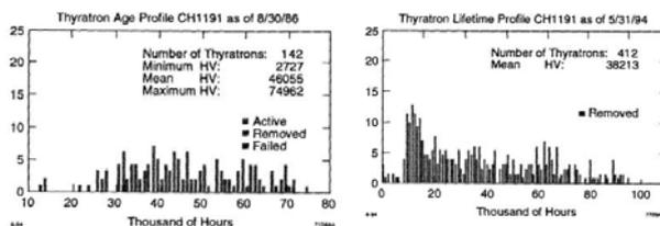
Figure 7. The quantity of tubes versus the high-voltage running-time hours.
